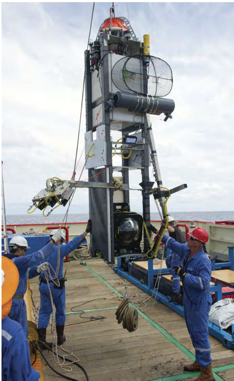
Figure 1. The DEEPSEA CHALLENGE Alpha Lander, DOV MIKE , is lifted by crane during deployment. Photo by Charlie Arneson, used with permission, Earthship Productions.
