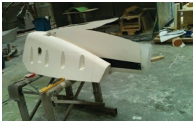
Figure 5. DSC stabilizer fin and triplet sub-assembly. Photo by Bruce Sutphen, used with permission, Earthship LLC.
