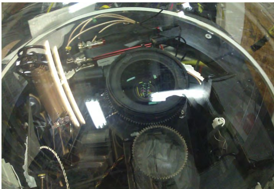
Figure 2. A Canon 5D camera is seen through the optically polished Nautilus Marine Vitrovex glass housing. Photo by Charlie Arneson, used with permission, Earthship Productions.
