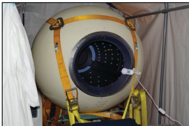
Figure 4. DSC pressure hull with interior view of carbon fiber plastic inner shell. Photo by Ron Allum. Used with Permission, Earthship LLC.
