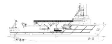
The Submarine Support and Rescue Vessel (SSRV) is designed to carry out rescue for a distressed submarine in rough weather up to sea state 5. Through the Public Private Partnership, ST Marine was awarded the contract to Design, Build, Own and Operate the SSRV - the first of its kind developed to meet the operational requirements of the Republic of Singapore Navy.
