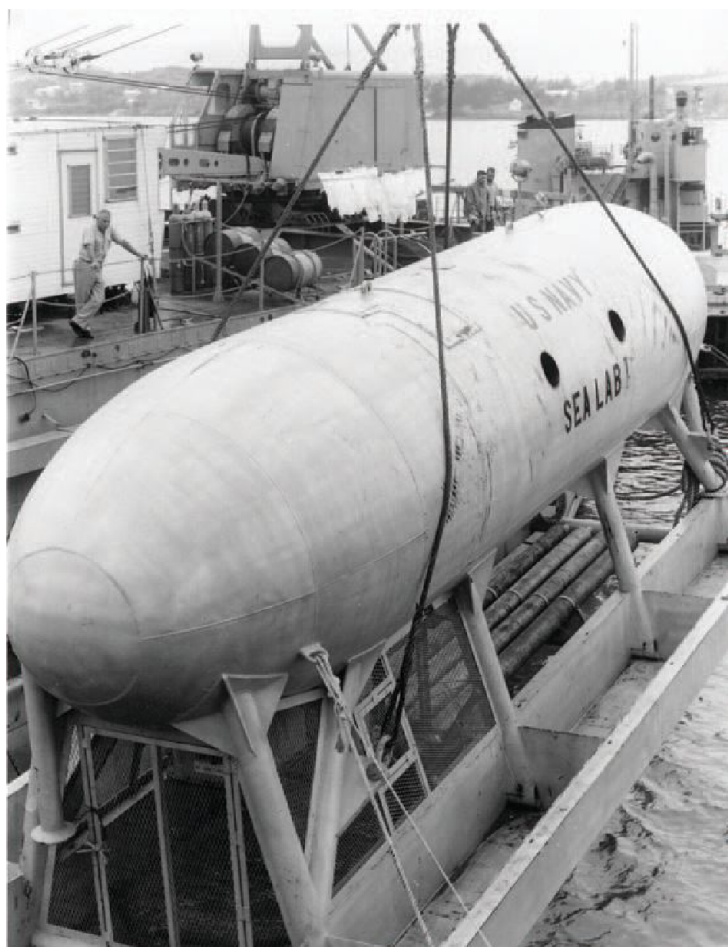
SEALAB I was a 40' x 9' cylinder without windows. Photo credit: U.S. Navy.
